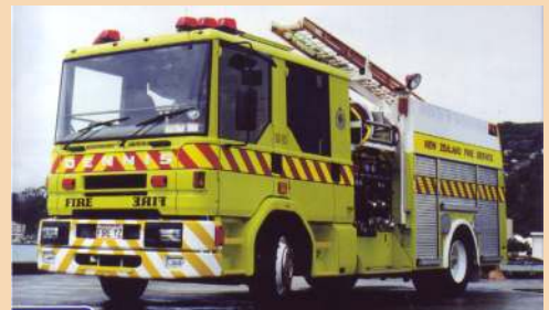
DENNIS • REG No: FIREYZ • Year: 2001 • Pump Output: 65 litres per second • Water Tank Capacity: 1,350 litres • Engine Power Output: 221kw @ 2200rpm • Weight: 13,080kg
