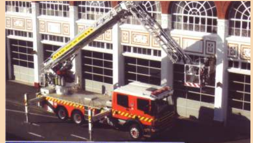
SCANIA - Aerial Appliance, Pump Elevating Platform • REG No: X05953 • Year: 1998 • Pump Output: 97.5 Litres per second • Engine Power Output: 300HP • Weight: 22,120kg • Aerial Component: Bronto 32PDT
