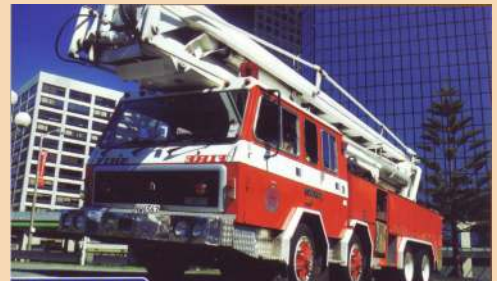
INTERNATIONAL Hydraulic Elevating Platform • REG No: MW6563 • Year: 1988 • Pump Output: 112 litres per second • Engine Power Output: 261kw @ 2100rpm • Weight: 21,500kg
